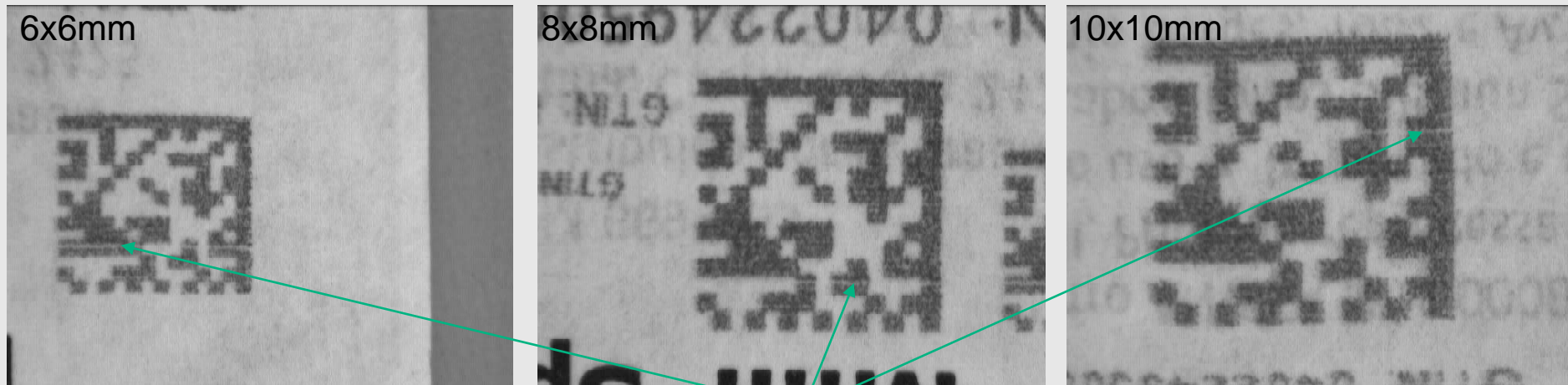
Lines caused by blocked nozzles
